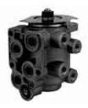
\*Overall height: 5-1/16" Rear ports: (4) 1/2" Side Ports: (8) 1/4" Mounting Studs: (3) 1-1/2" L Replaces: Bendix 286773 (E-7)
